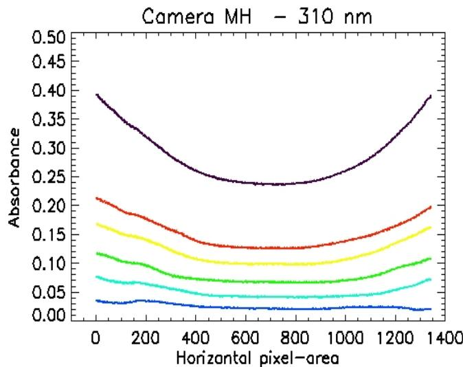
Calibration cell A25 ( $\sim$ 1600ppmm) - at 09:17 LT  $\tau_{A_{\text{SO}_2} + \text{glass}} = 0.335$
