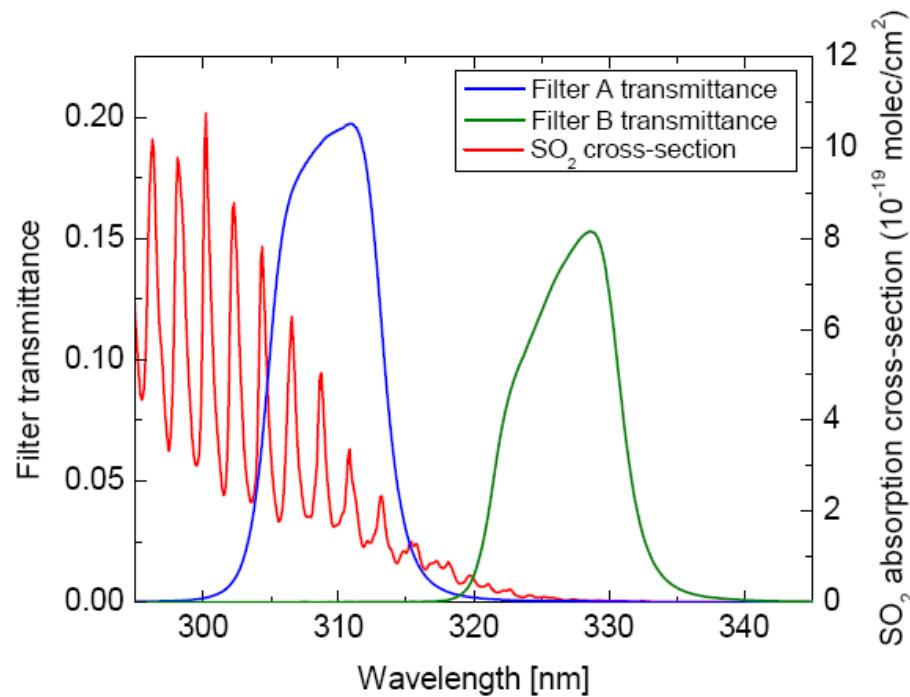
**Fig. 4.11 – Measured transmittance of the two band-pass filters used for construction of the  $SO_2$ -camera prototype. Also shown (red) is the absorption cross-section of  $SO_2$  (Bogumil et al. 2003). (Adapted from Kick 2008)** **[from Kern, AMTD, 2010]**
