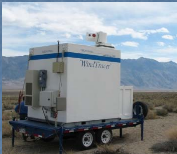
Windtracer DWL Lockheed Martin and vertical cross section of Doppler lidar
