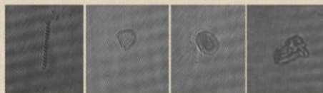
Fig. 3. Holograms for transparent atmospheric aerosols from different samples (days) belonging to the four main classes a) wire, b) column, c) spherical fragments, d) irregular
