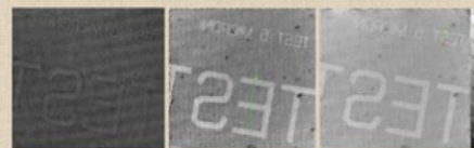
Fig. 2. a) Hologram and b, c) reconstruction for the object fabricated by e-beam lithography for system calibration (25µm in b and 5µm in c)
