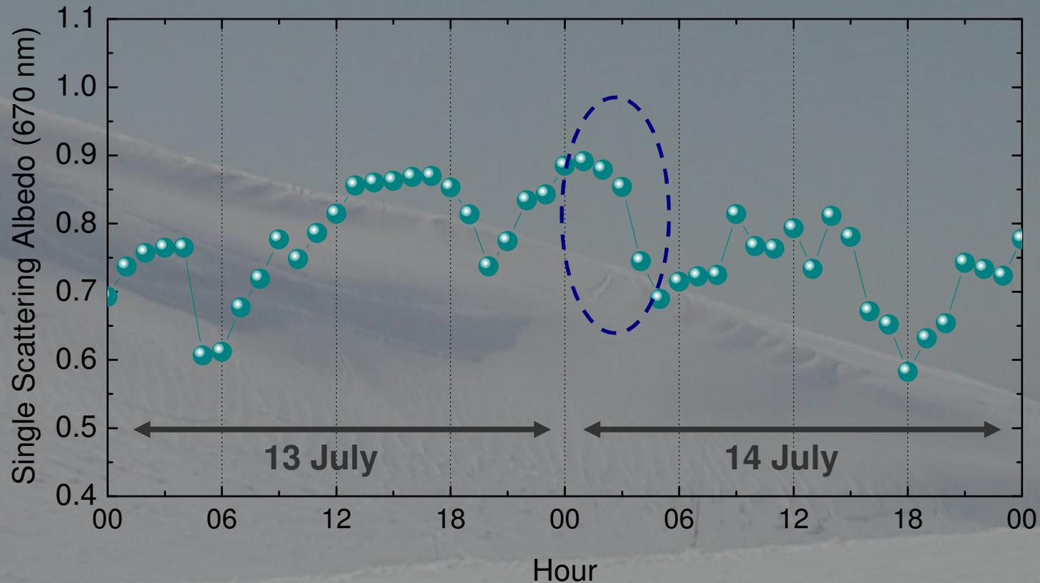
Single scattering albedo determined by TSI nephelometer and Multi Angle Absorption Photometer (MAAP)
